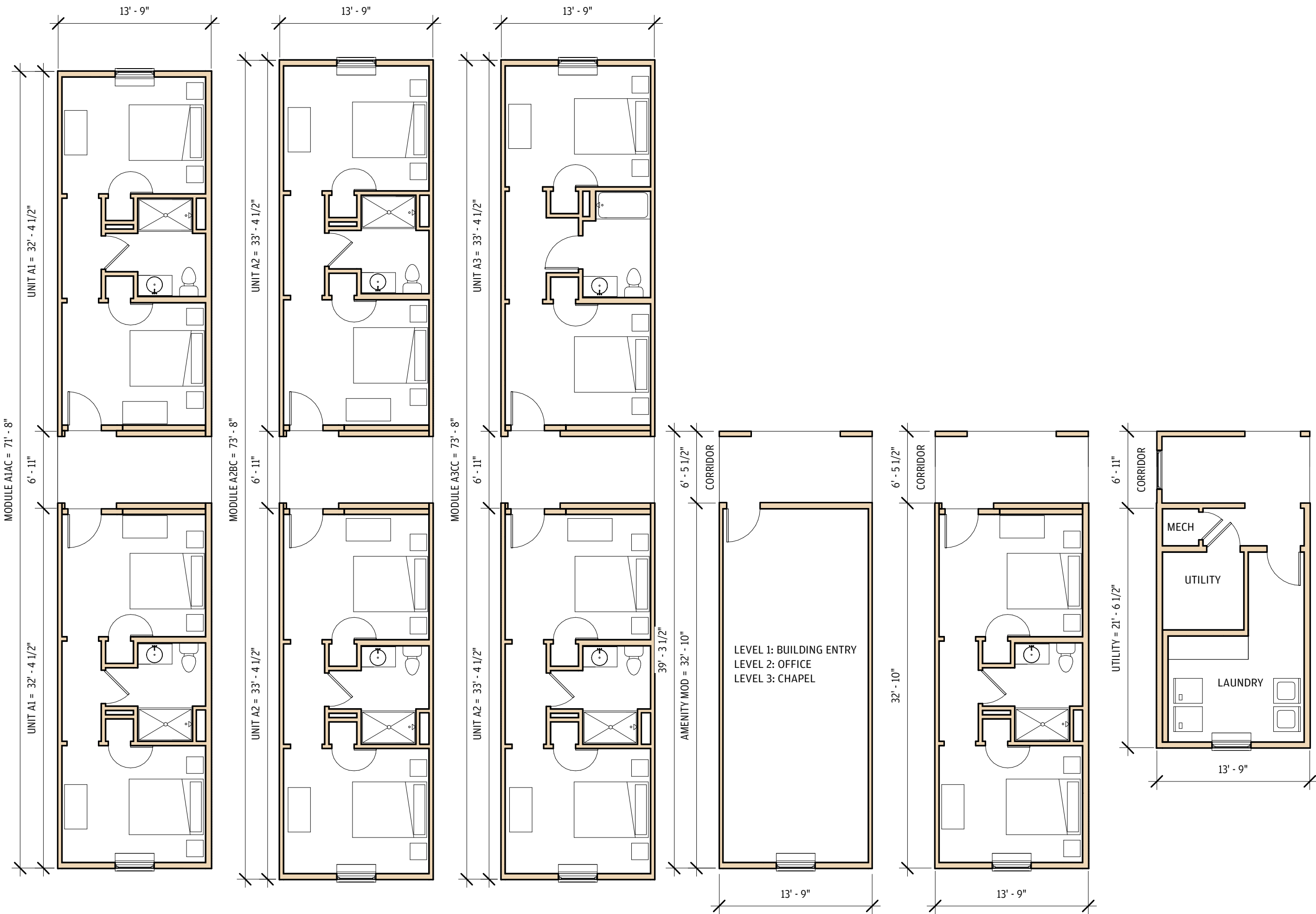
1 MODULAR PRODUCTION LINE ROLLS - ARCHITECTURE 1/8" = 1'-0"
